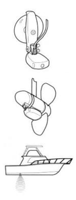
Thru-hull mounting may require the use of a fairing block to level the transducer with the waterline. Also, since special tools and knowledge may be required to perform this type of installation, it is best to refer to a qualified marine technician.
